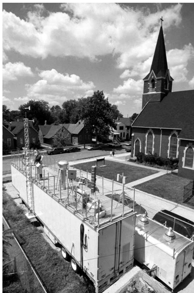
Figure 2. The mobile air research laboratory (AirCARE 1). Note the ambient air monitoring equipment mounted on top of the trailer.
